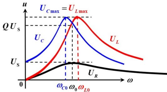
$$U_R = IR = \frac{U_s}{\sqrt{1+Q^2\left(\frac{\omega}{\omega_0} - \frac{\omega_0}{\omega}\right)^2}}$$
